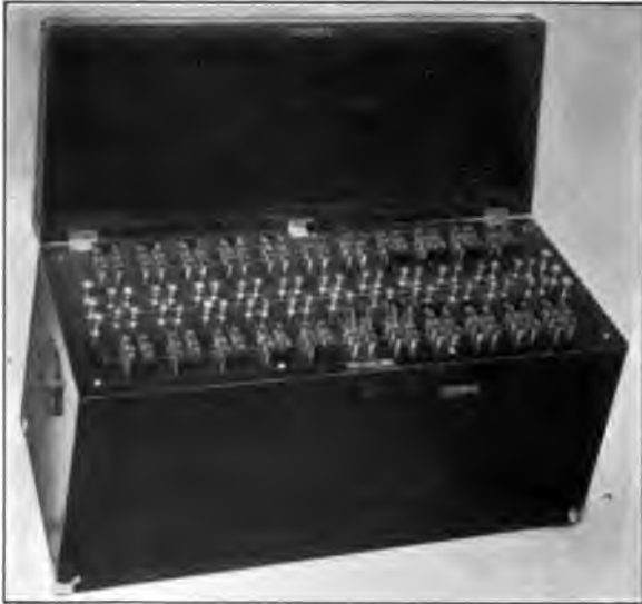
FIG. 126A.—Western Electric Company's artificial aerial telephone line ward, and cuts it out of circuit when thrown outward. As connected in Fig. 127, there is one section of 2 miles (3.2 km.) left inserted in the line. By selecting the proper combination o
